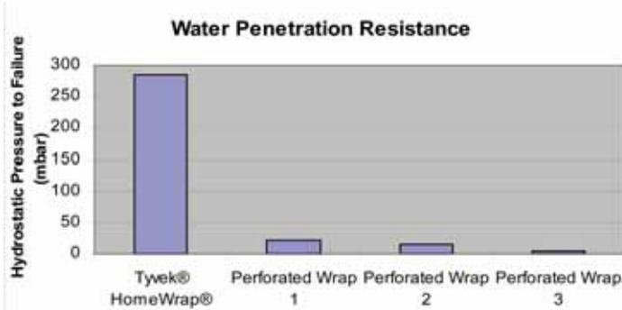
The ability of a housewrap to hold out bulk water is one of the most basic and important requirements of any weather resistant barrier. DuPont Tyvek® HomeWrap® has over 13 x Greater water holdout than perforated housewraps, as tested in accordance with the Hydrostatic Head Test (AATCC-127). Tyvek® HomeWrap® passed the high duty water holdout requirements ASNZ 4201.4
