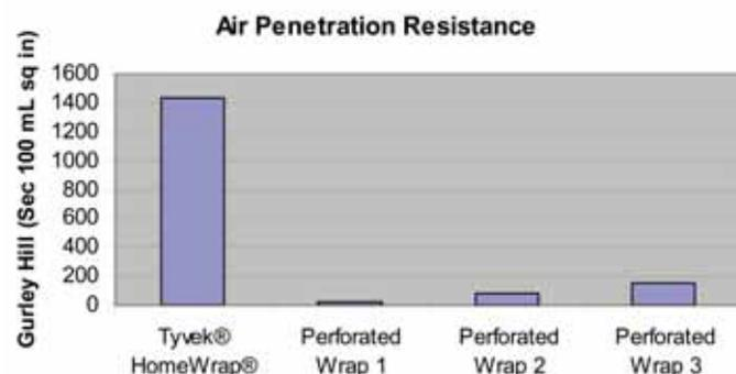
Tyvek® HomeWrap® has higher air resistance than perforated housewraps.
