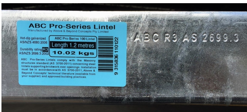
ABC Pro-Series Lintels are metal stamped before hot-dip galvanizing and are labelled before packing
